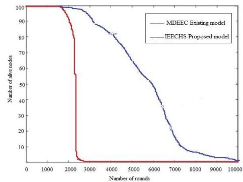
Fig. 6: Number of Alive Nodes for 100 x 100 m2
