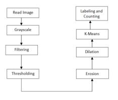
Figure 1 Block diagram of the proposed methodology
