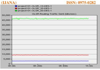
Figure 3.3: Routing overhead in OLSR and TORA for 10, 20 and 50 nodes
