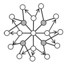
Fig. 1.1 Multipoint Relays (MPRs) are in gray colour. The transmitting node is shown at the center of the sample structure
