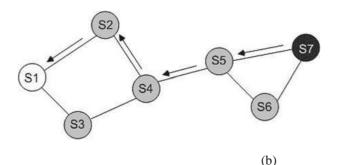
Figure 1.2 AODV protocol (a) Source node broadcasting the route request packet. (b) Route reply is sent by the destination using the reverse path
