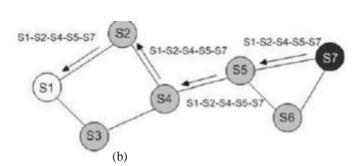
Fig. 1.3 (a) Route Discovery (b) Using route record to send the route reply
