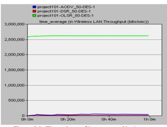
Figure 3.9: Throughput -50 sources at 30m/s
