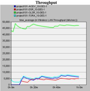
Figure 3.8: Throughput -10 sources at 10m/s, 20 sources at 30m/s
