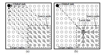
Fig 1: Data gathering of two methods in a geographic routing(a)datagathering without a local sink and (b) data gathering with a local sink
