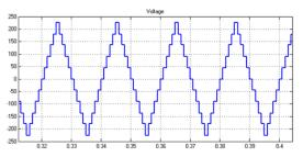
Fig.3. Multilevel inverter line output voltage waveform.
