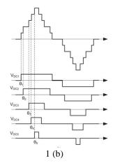
$$V_{\text{fund}} = \frac{4}{\pi} (V_{\text{dc1}} \cos (\theta_1) + V_{\text{dc2}} \cos (\theta_2) + \dots + V_{\text{dc5}} \cos (\theta_5))$$
