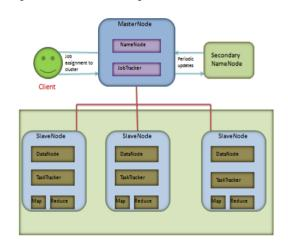
Figure 5: Hadoop Distributed File System Architecture
