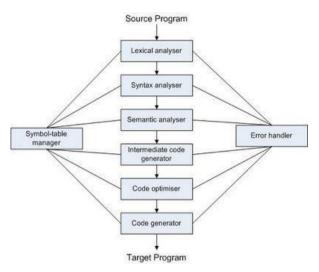
Fig: 2.1 structure of a compiler [1]
