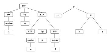
Fig: 3.6 Example for Syntax analysis
