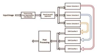
Fig. 5. Block diagram of the proposed CR system
