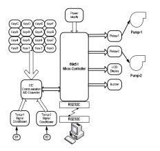
Fig 3.1 TMCNRS Hardware Integration diagram
