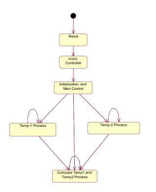
Figure 4.11 Top Level state diagrams
