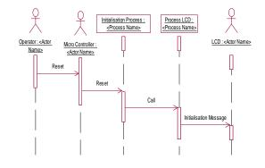
Fig 4.5 Sequence Flow for the Event "Push Reset button"
