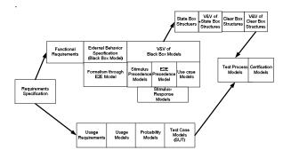
Fig 1.2 Refined CRSE for formalizing the External behavior of the embedded system
