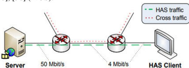
Figure 4: Overview of the simulated topology. [5]
