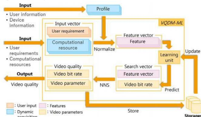
Figure 8: The Video quality determining mechanism with machine learning. [19]
