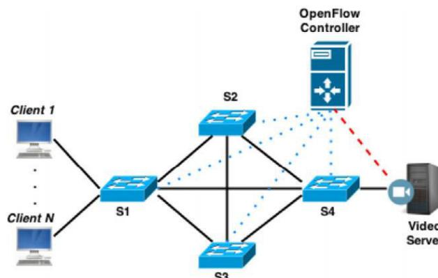
Figure 3: Network topology used in the simulations. There are six clients, one server and one controller in the network. The blue dotted lines indicate the OpenFlow protocol and the red dashed line represents the communication between the server and the controller. [31] A (frequency adjusted) Q-learning HAS client is proposed in [5]. The proposed HAS client dynamically learns the
