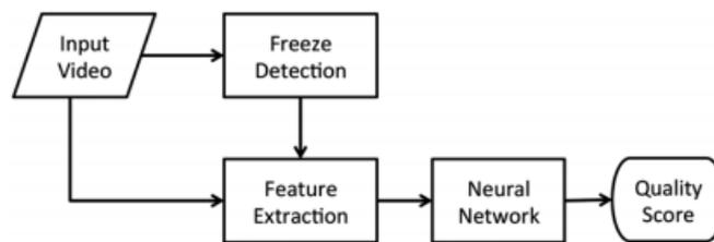
Figure 12: Flowchart of the proposed metric. [42]
