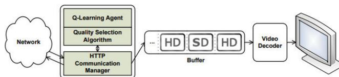
Figure 2: Schematic overview of the Q-learning HAS client design. [4]
