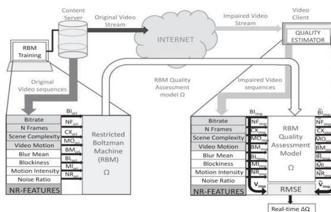
Figure 10: Real-time UDL-based video quality assessment method. [34]
