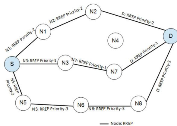
**Figure 6. PALBMRP Route Reply Process**
