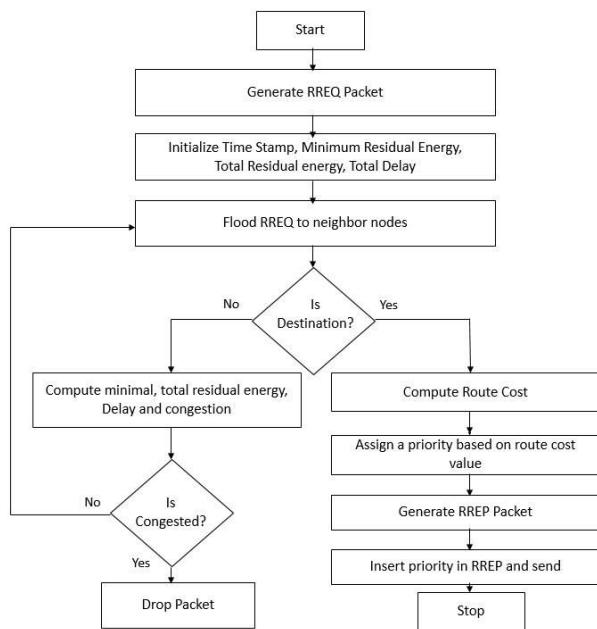
**Figure 3. Route Request Reply Traversal Flow Chart**
