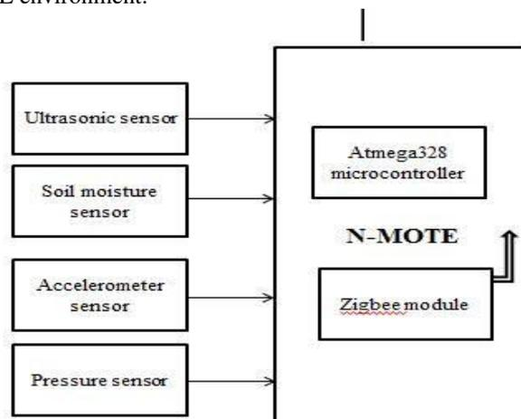
Fig 1. Transmitter Circuit.
