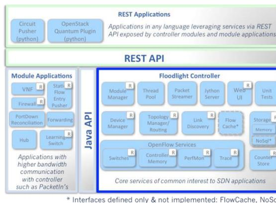
Fig. 3. Floodlight controller structure [11]
