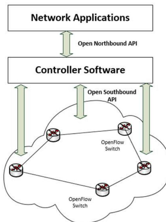
Fig. 2. Simplified view of the SDN architecture.
