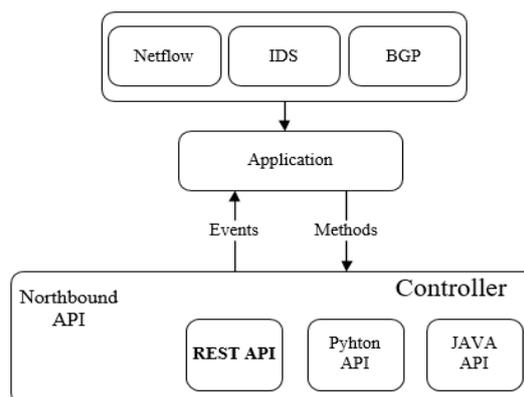
Fig. 4. SDN controller northbound API
