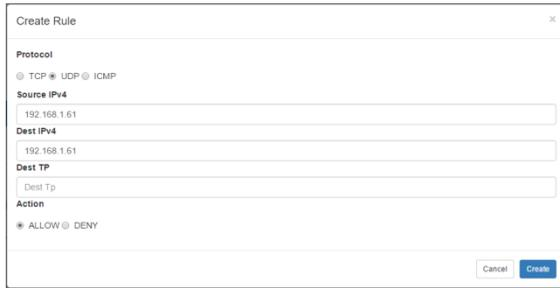
Fig.9. Adding a record to the ACL
