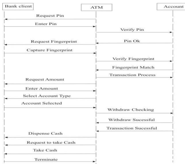
Fig. 2. Activity diagram of the proposed prototype
