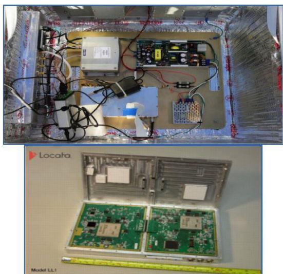
Figure 1: (a) LocataLite inside box with cabling to antennas, and (b) Locata receiver box.
