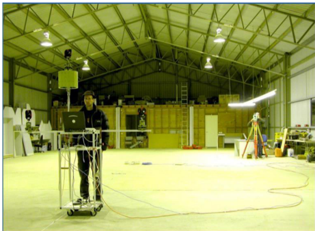
Figure 5: Indoor test site, Locata receiver on trolley and RTS set-up.
