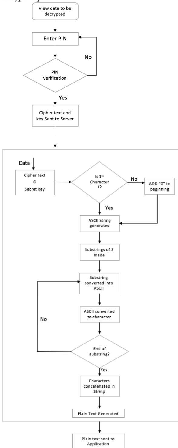
Figure 2. Flowchart for decryption algorithm
