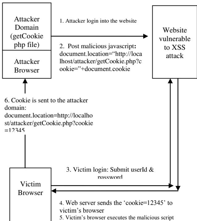
Fig.1 The architecture for exploiting XSS vulnerabilities
