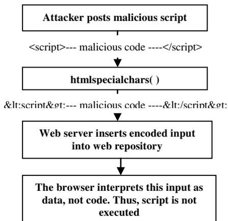
Fig.2 Flow chart for encoding
