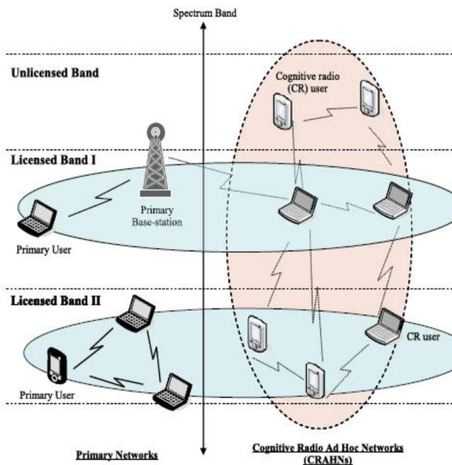
Figure 2. The CRAHN architecture
