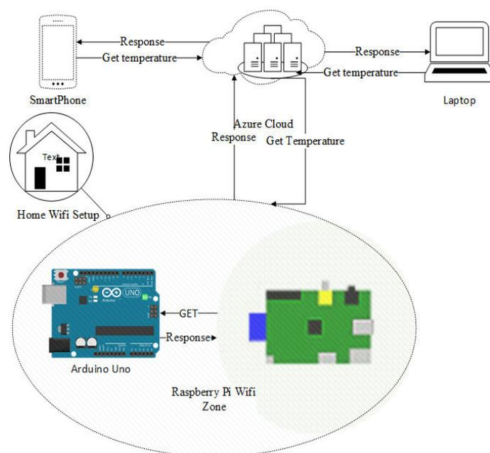
Fig 1. Network topology diagram of WoT devices
