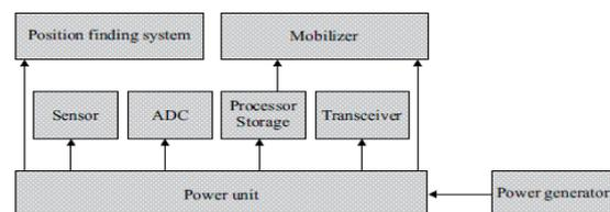
Fig. 2: Sensor node Architecture
