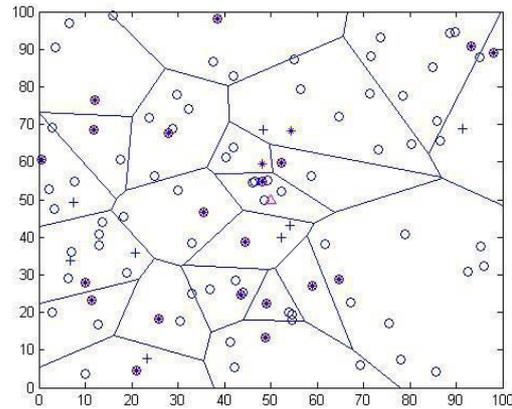
Fig. 6: Clustering of Sensor Nodes
