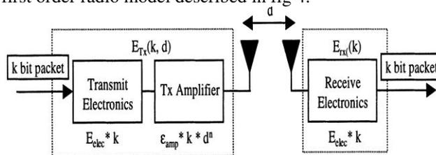
Fig4: Radio energy dissipation model
