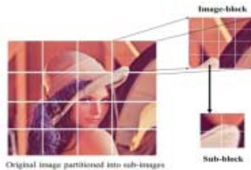
Fig. 5: Definition of sub-image and image-blocks
