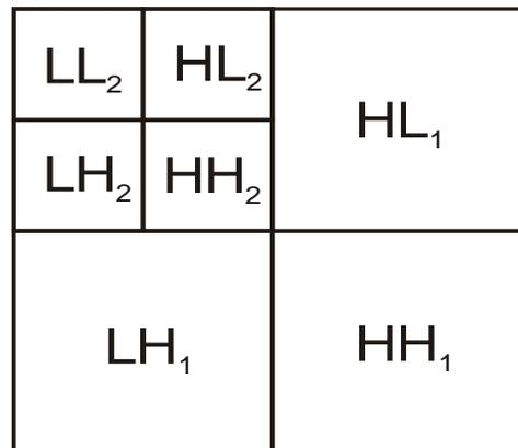
Figure Scale 2-Dimensional Discrete Wavelet Transform
