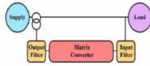
Figure 2.2 Matrix converter based DVR.
