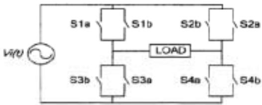
Fig 4.2 Single-phase matrix converter circuit configurations at load
