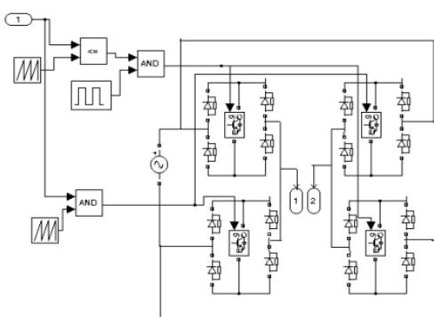
Figure 6.3 Subsystem 2 of the Closed loop DVR with a matrix converter
