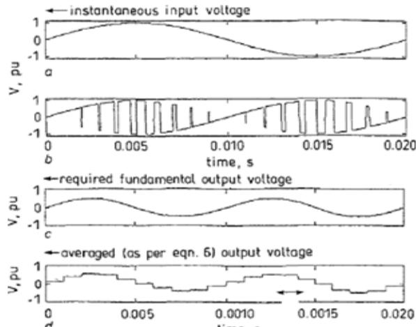
Fig 4.3 Input, Output, required output and averaged output wave forms
