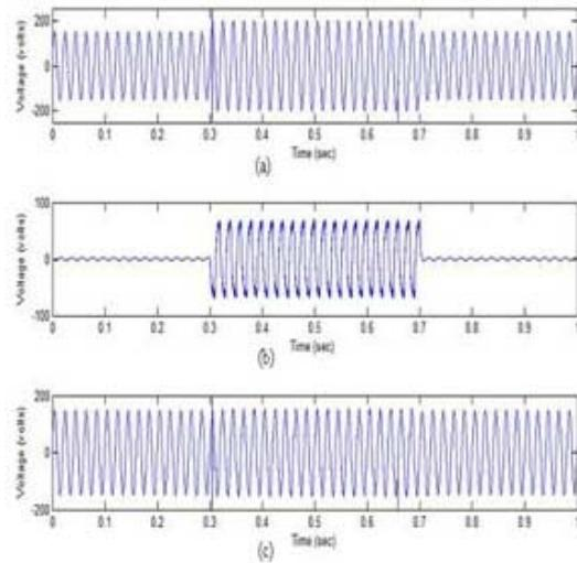
Figure 6.5 Response of RMC based DVR to a voltage swell
