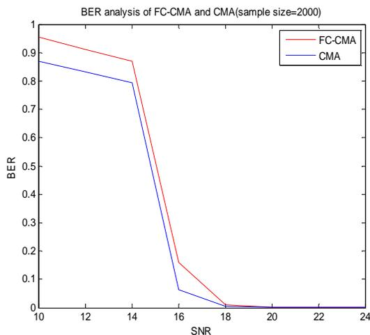
**Figure 4.1:** Plot of the BER Vs SNR using CMA and FS-CMA.
