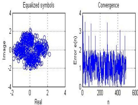
Figure 2.1 Symbol equalization Figure 2.2 MSE Convergence when Maximum sample size is 500 and SNR = 10 Db
