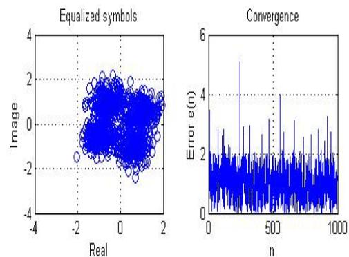
Figure 2.5 Symbol equalization Figure 2.6 MSE Convergence when Maximum sample size is 1000 and SNR = 10Db
