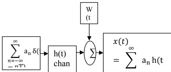
**Figure 1.2:** Block diagram of Channel model for a 4-QAM source.
