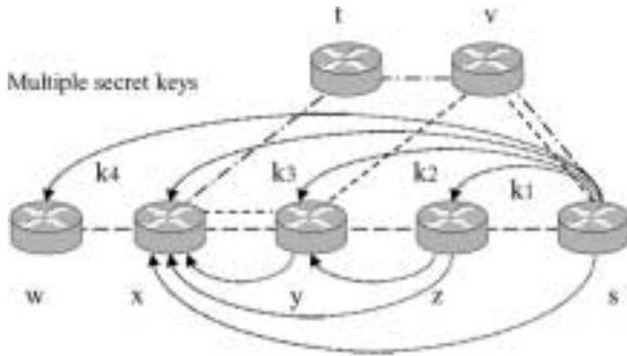
Fig.1. Multiple secret keys are shared between a source and the intermediate nodes and the destination node.
