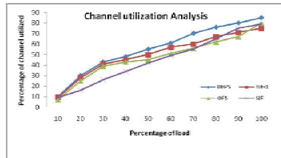
Figure 6: Graph showing the comparison of percentage of Channel utilized using DFPS Algorithm versus conventional Algorithms
