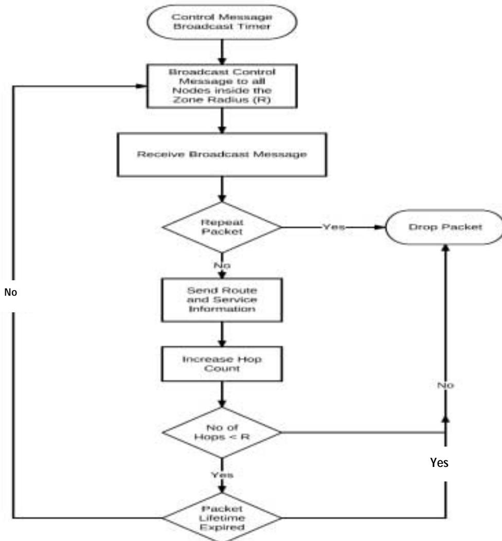
Fig1. Broadcast Mechanism
