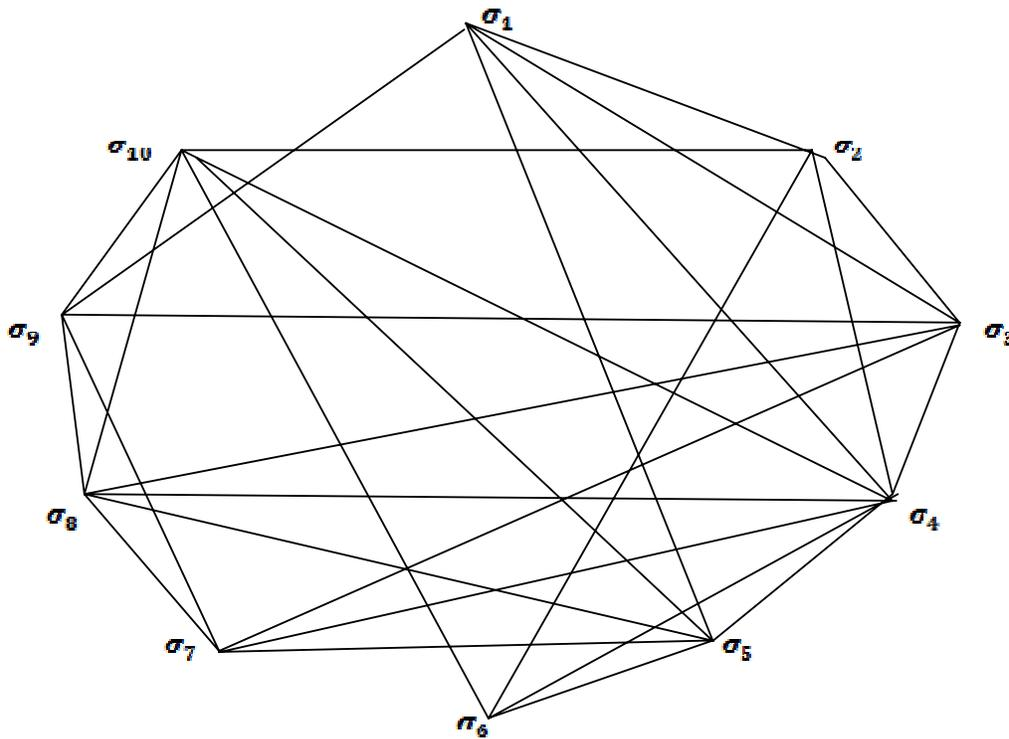
Fig. 6.3 : Compatibility Graph of the intersection (Fig. 6.1) when left turn of traffic stream  $\sigma_3$  is allowed
