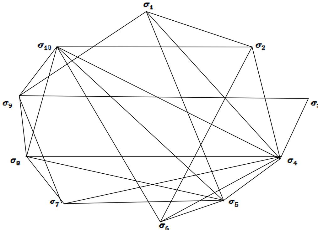
Fig. 6.2 Compatibility Graph of the intersection ( Fig. 6.1 )
