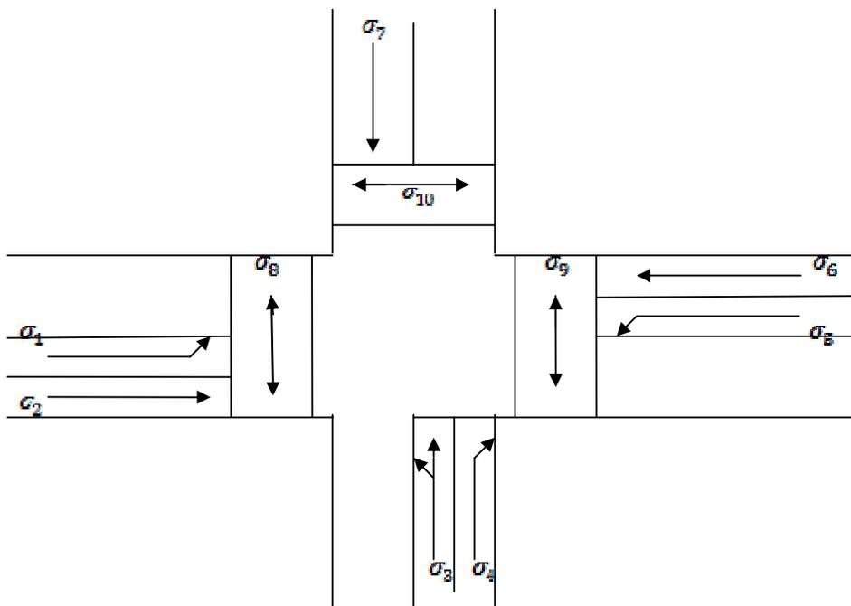
Fig. 6.1 : An intersection with ten traffic streams
