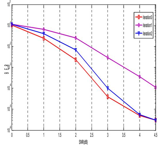
Fig. 3 BER Performance of turbo Log-MAP based MUD with code rate 1/2.
