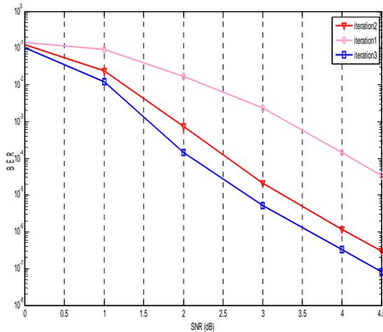
Fig. 4 BER Performance of turbo Log-MAP based MUD with code rate 1/3.
