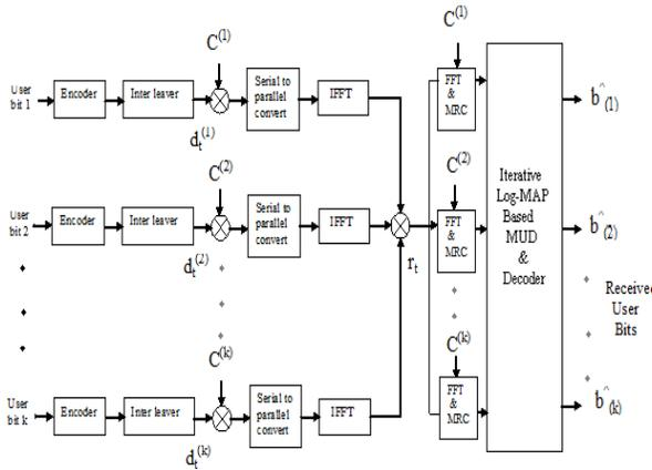
Fig. 1 Coded MC-CDMA system model
