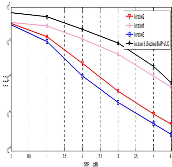
Fig. 5 comparison of proposed Log-MAP based MUD with optimal MAP based MUD.
