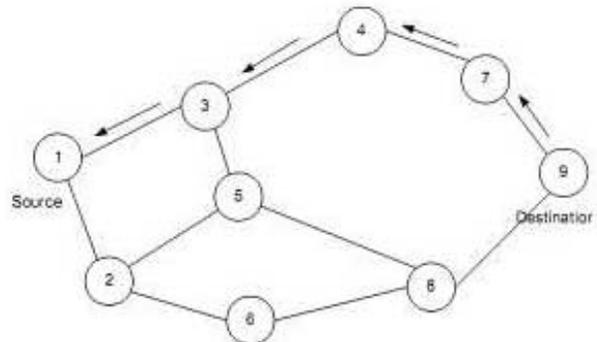
Fig 4: The forwarding of Route Reply packet in AODV
