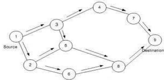
Fig 3: The Route Request packets flooding in AODV
