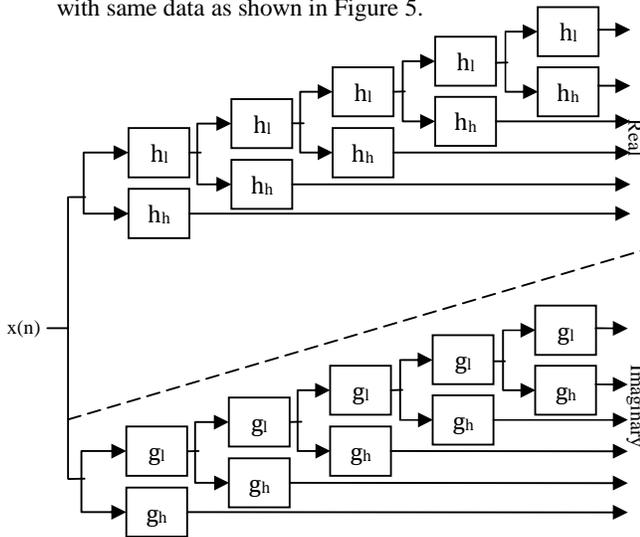
Fig.5. Filter Bank of DT-CWT
