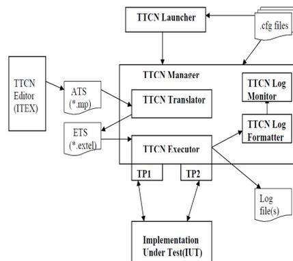
Fig. 2:TTCN-2 test system
