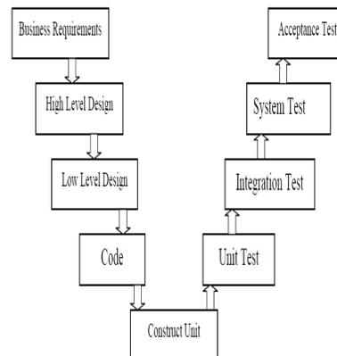
Fig. 1: Test phases in relation with development phases V-Model
