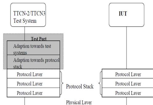
**Fig. 4: Conceptual view of test port**
