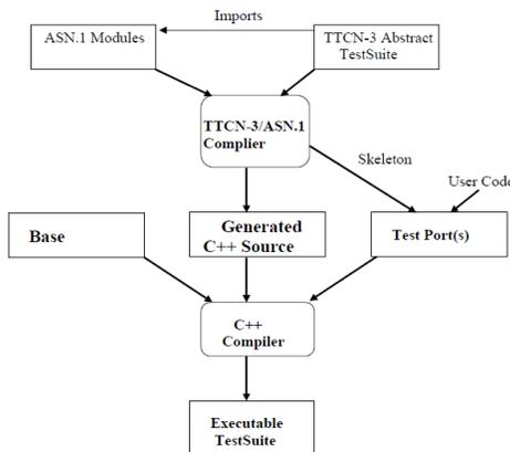
**Fig. 3:Structure of TTCN-3 EXECUTER**
