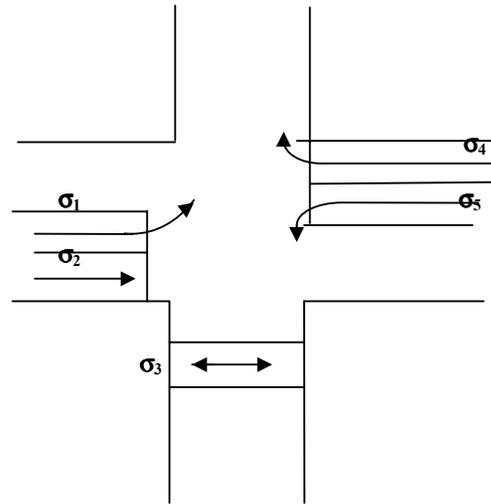
Fig. 5.1 : An intersection with five traffic streams.
