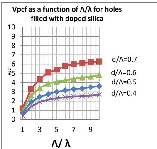
Fig.4(b): Effective V parameter for different values of  $d/\Lambda$  in proposed PCF
