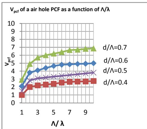
Fig.4(a): Effective V parameter for different values of  $d/\Lambda$  in Air-Hole PCF
