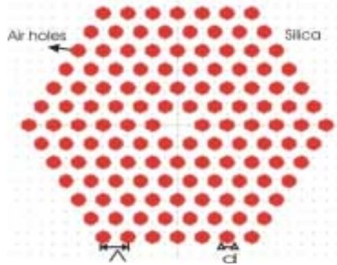
Fig.1: Conventional Photonic Crystal Fiber
