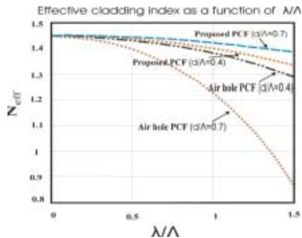
Fig.5: Effective refractive index of conventional PCF and proposed (doped silica rods in cladding region)PCF for different values of  $d/\Lambda$ .
