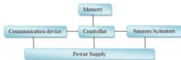
Figure 2: Overview of main sensor node hardware components
