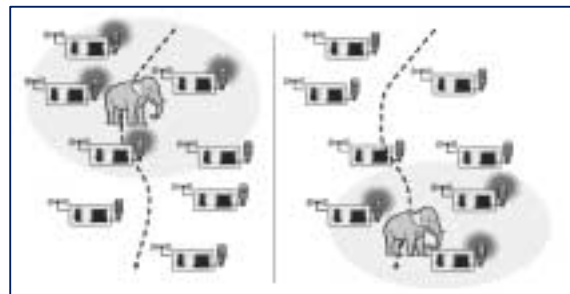
Figure 8 Area of sensor nodes detecting an event – an elephant – that moves through the network along with the event source (dashed line indicate the elephant's trajectory; shaded ellipse the activity area following or even preceding the elephant)
