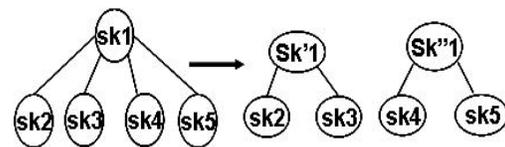
Fig 7: Node  $sk_1$  splits into nodes  $sk'_1$  and  $sk''_1$ . B-tree order  $m=3$ .
