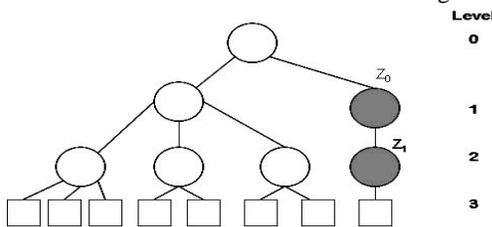
Fig.8: An NSBHO tree of order 3. The shaded nodes are in the special path (SP). The tree height  $h=3$ (the external nodes are excluded).
