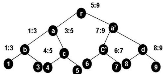
Fig 5: continues (c) 2-3 Tree after inserting 4 in 5a.
