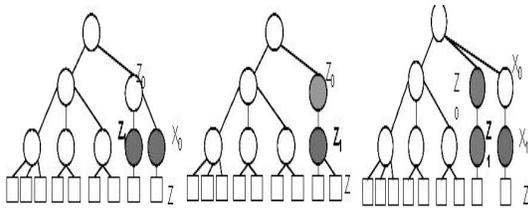
**Fig.9: An external node z is inserted into the NSBHO tree specified in 4.1 using the insertion point. (a) z<sub>0</sub>, (b) z<sub>1</sub>, (c) root. The resulting trees at (a) and (c) are not NSBHO trees. The resulting tree at (b), however, is an NSBHO tree.**
