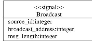
**Figure 5 UML Class Diagram of Broadcast**
