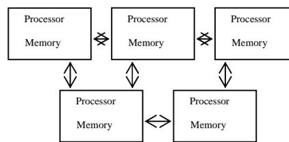
**Figure 1 Structure of Distributed Computer System**
