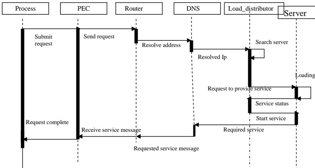
Figure 7 UML Sequence Diagram of Process Request
