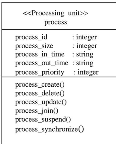
**Figure 3 Class Diagram of Process**
