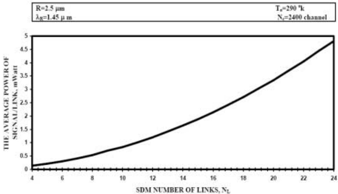
Fig. 7. Variations of  $P_{s,ave}$  against variations of SDM number of links at the assumed set of parameters.
