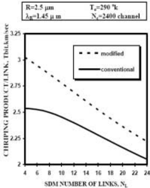
Fig.5. Variations of chirping product/link, Tbit.km/sec against variations of SDM number of links at the assumed set of parameters.
