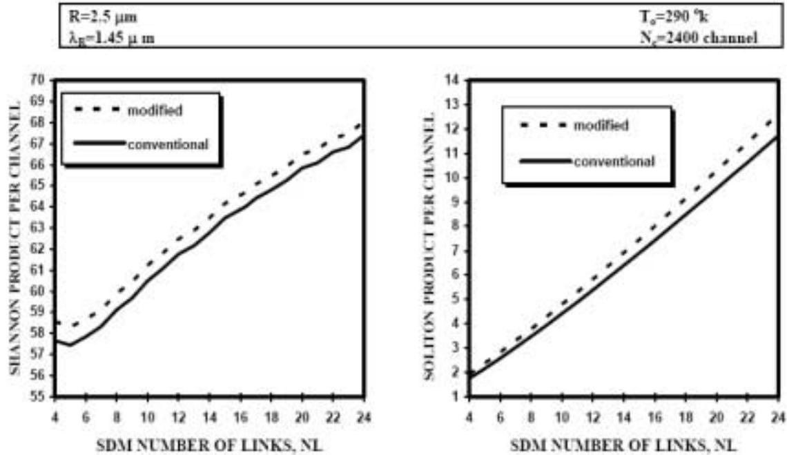
Fig.8. Variations of Shannon product/channel, Tbit.km/sec against variations of SDM number of links,  $N_L$  at the assumed set of parameters
