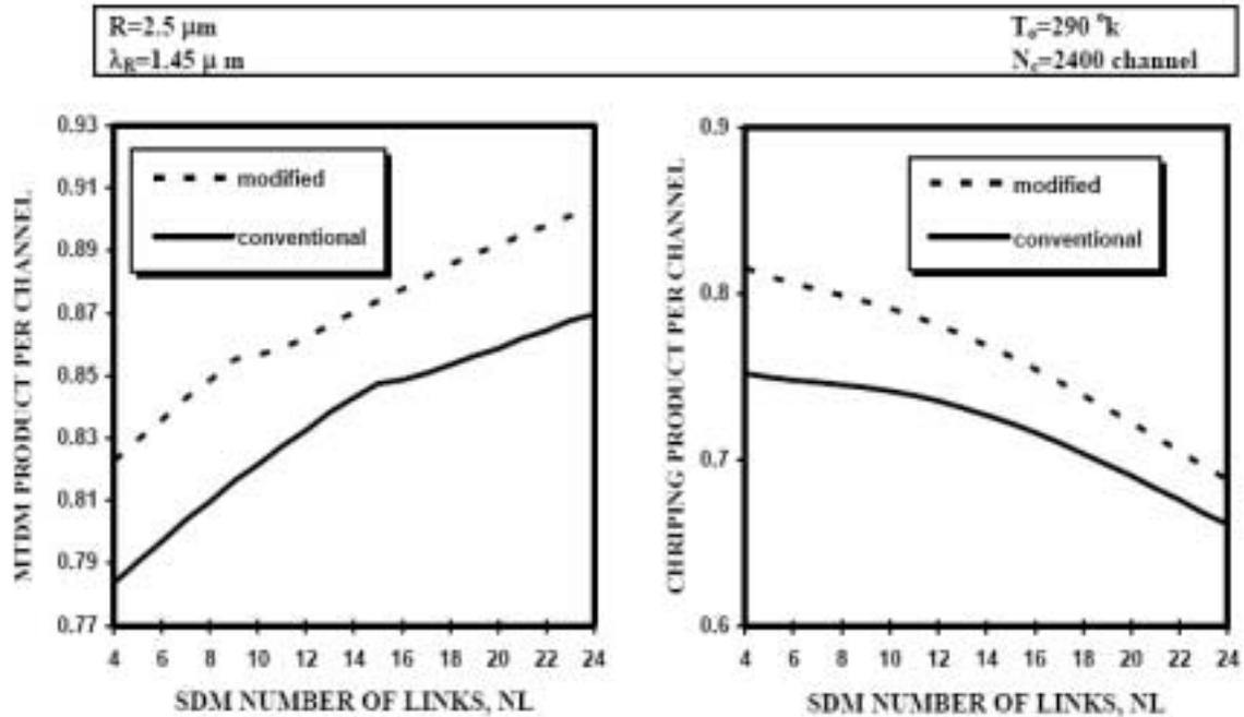
Fig.10. Variations of MTDM product/channel, Tbit.km/sec against variations of SDM number of links,  $N_L$  at the assumed set of parameters
