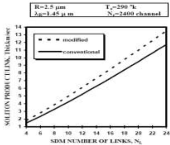
Fig.4. Variations of soliton product/link, Tbit.km/sec against variations of SDM number of links at the assumed set of parameters
