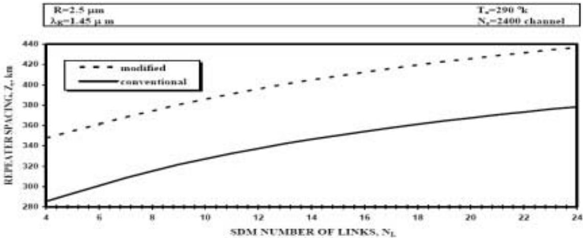
Fig. 2. Variations of repeater spacing against variations of SDM number of links at the assumed set of parameters.
