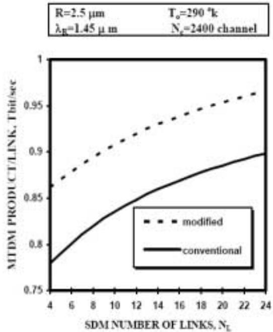
Fig.6. Variations of MTDM product/link, Tbit.km/sec against variations of SDM number of links  $N_L$  at the assumed set of parameters
