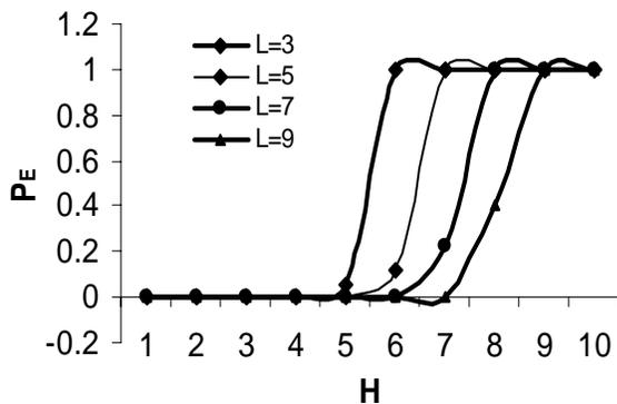
**Fig. 4:** Success probability of the Majority Flipping Attack as a function of H. Symbols denote the simulations results for  $K = 3, Y=3, Z=3, \eta=3, M = 100$  and  $N = 1000$  ( $H = \eta + 0.45 * L$ ).
