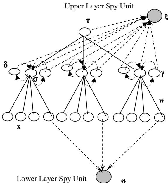
**Fig. 1: A structure of Tree Parity Machine with K=3, Y=3, Z=3,  $\vartheta=1$ ,  $\xi=1$  and N=4.**
