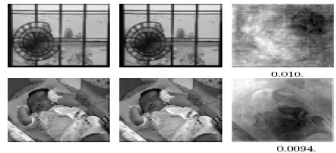
Figure 5: Images in left column are the original, middle are the respective watermarked image and right are the differences. The differences are enhanced (by scaling the intensity) for better printing quality. The values below the images are the distortion.
