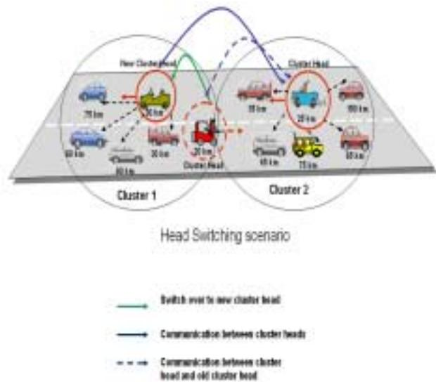
Figure 3: Head switching process
