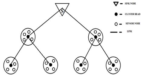
Figure 1: Structure of point to multipoint WSN
