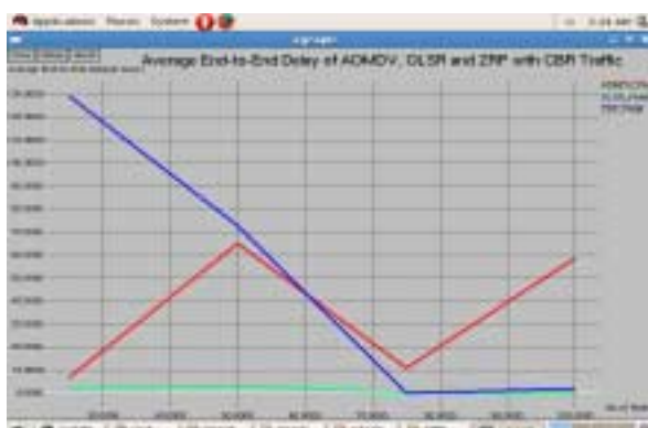
Fig. 39. e2e delay of AOMDV, OLSR and ZRP with CBR Traffic in PMM
