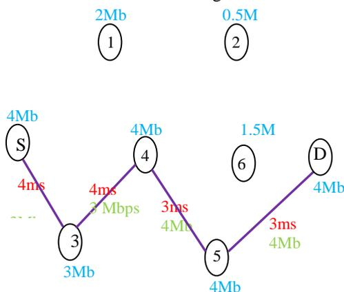
**Fig. 3 Optimum path from Node S to Node D**
