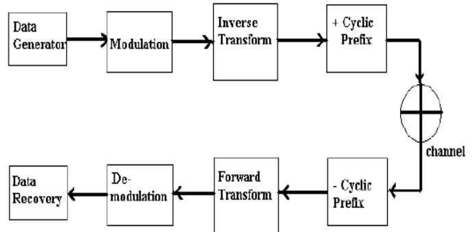
Figure 1. Basic block diagram of FFT based OFDM [2]
