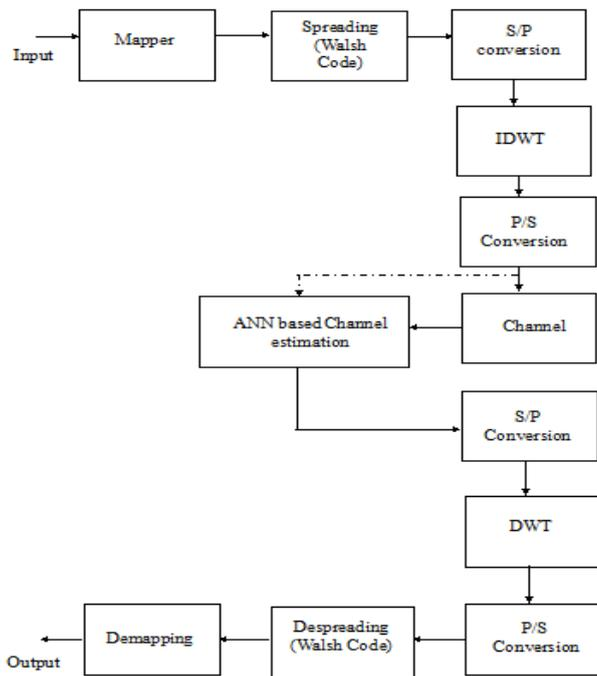
Figure 4. DWT based OFDM using ANN Channel
