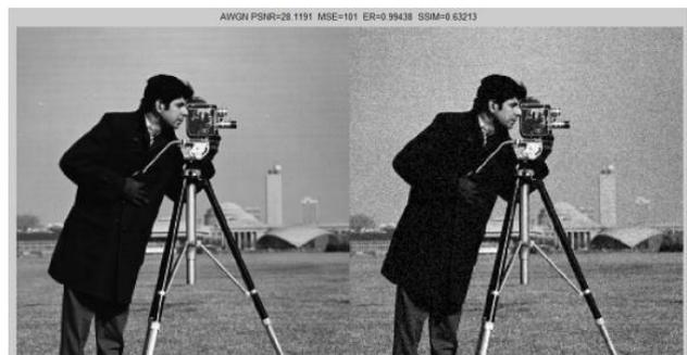
Figure 2 Original Image Vs AWGN Noisy image
