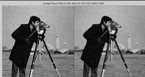
Figure 4 AWGN Noisy Image Vs Average Filter output
