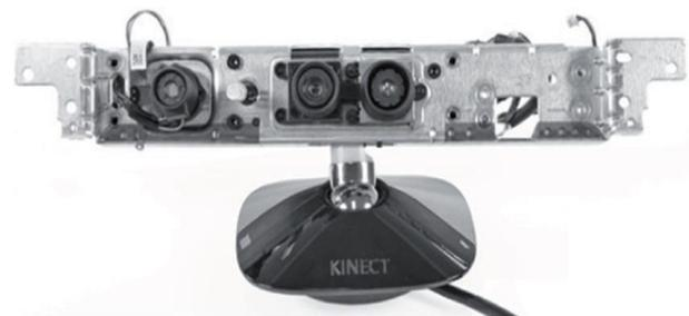
**Figure 1** The infrared (IR) projector, IR camera, and RGB camera inside a Kinect sensor.
