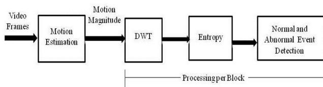
Fig. 1: Proposed approach block diagram
