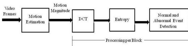
Fig. 2: DCT- Block based processing framework
