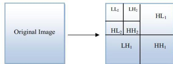
Figure 1: Two level DWT decomposition
