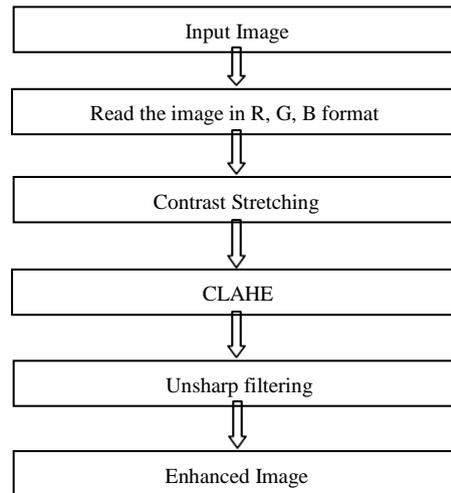
Fig. 1: Flow Sequence of the Proposed Method
